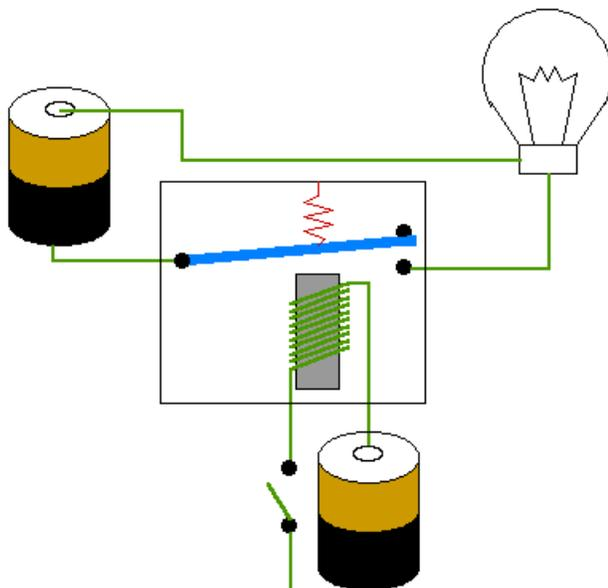
In this bottom left figure, you can see that a relay consists of two separate and completely independent circuits. The first is at the bottom and drives the electromagnet. In this circuit, a switch is controlling the power to the electromagnet. When the switch is on, the electromagnet is on, and it attracts the armature (blue). The armature is acting as a switch in the second circuit. When the electromagnet is energized, the armature completes the second circuit and the light is on. When the
