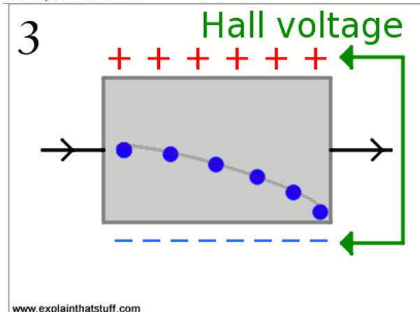
3. Now looking from above, the electrons in this example would bend as shown. With more electrons on the right side of the material than on the left, there would be a difference in potential (a voltage) between the two sides, as shown by the green arrowed line. The size of this voltage is directly proportional to the size of the electric current and the strength of the magnetic field.
