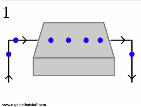
1. When an electric current flows through a material, electrons (shown here as blue blobs) move through it in pretty much a straight line.
