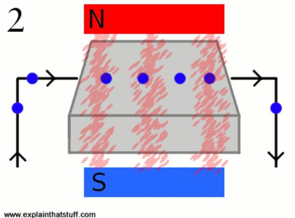
2. Put the material in a magnetic field and the electrons inside it are in the field too. A force acts on them (the Lorentz force) and makes them deviate from their straight-line path.
