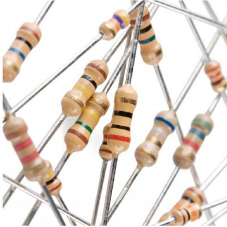
Through-hole, axial resistors usually use the color-band system to display their value. Most of these resistors will have four bands of color circling the resistor.
