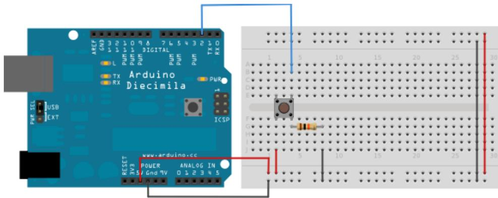
Connect three wires to the Arduino board. The first two, red and black, connect to the two long vertical rows on the side of the breadboard to provide access to the 5 volt supply and ground. The third wire goes from digital pin 2 to one leg of the pushbutton. That same leg of the button connects through a pull-down resistor (here 10 KOhms) to ground. The other leg of the button connects to the 5 volt supply.
