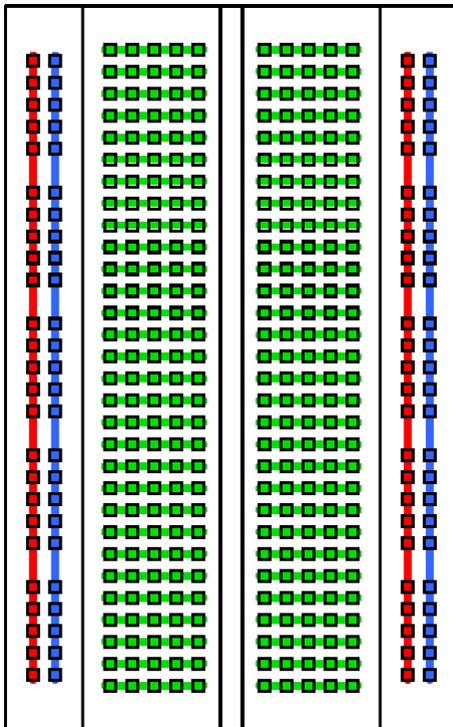
A breadboard is a construction base for prototyping of electronics. Originally it was literally a bread board, a polished piece of wood used for slicing bread. In the 1970s the solderless breadboard (AKA plug-board) became available and nowadays the term "breadboard" is commonly used to refer to these. "Breadboard" is also a synonym for "prototype".
